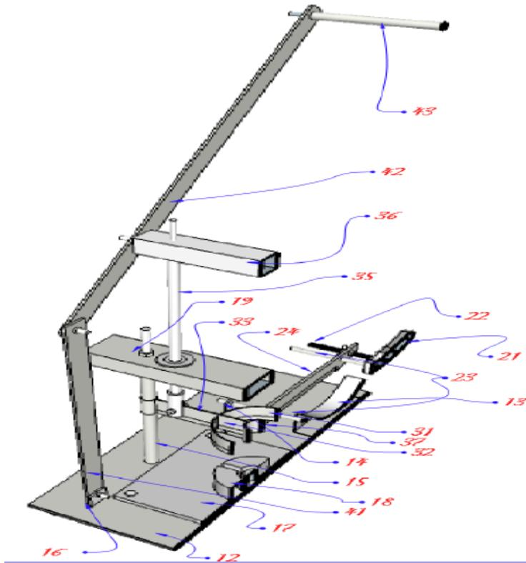
Figure 1. Cross-sectional view of the pineapple multiprocessing machine.
